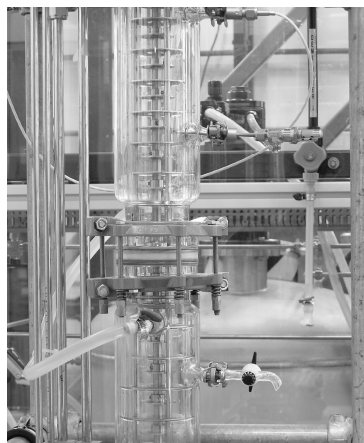
Figure 4. Scheme of a Rotating Disc Column ( www.liquid-extraction.com/rdc-column.htm ) and the actual pilot plant column.
